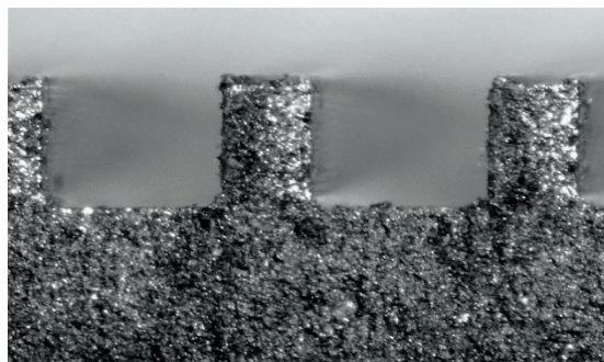
Figure 8: Cross-section microscope picture (X20) of uncoated microchannel substrate.
