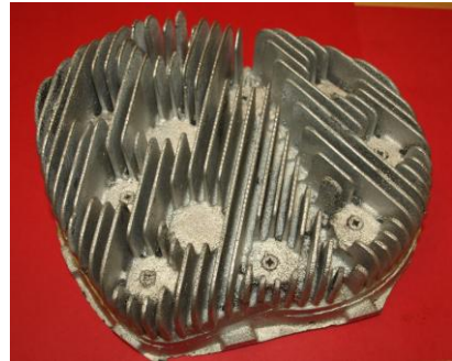
Figure 2: Engine head cast using aluminium
