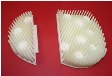
(a) ABS pattern printed in two parts
